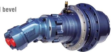
> **PWD and SLW Series Winch Drives** - Rotating housing planetary gearboxes with integrated brakes and various motor options. Torque ranges from 3,000 to 850,000 Nm. In drum design for compact winches. DNV type approval on these winches is available.
